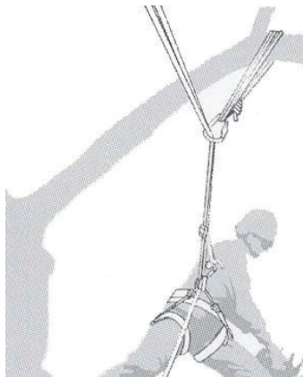
Figure A.3 – Example of redirection of main line via supplementary anchor point
